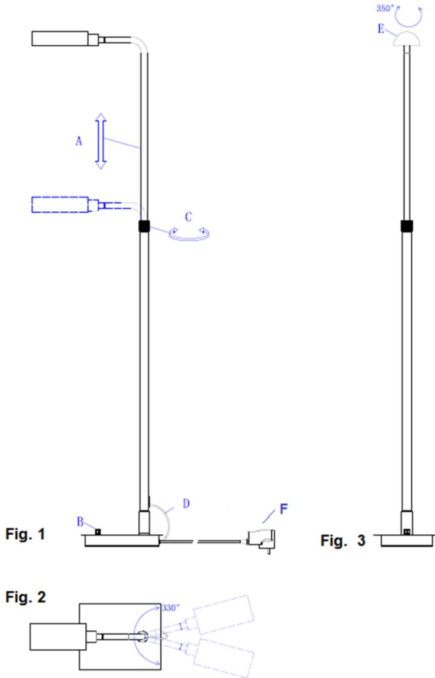
**NOTE:** When adjusting the head (E), do not adjust more than the degrees shown in above diagram, as this may damage the internal wires.
