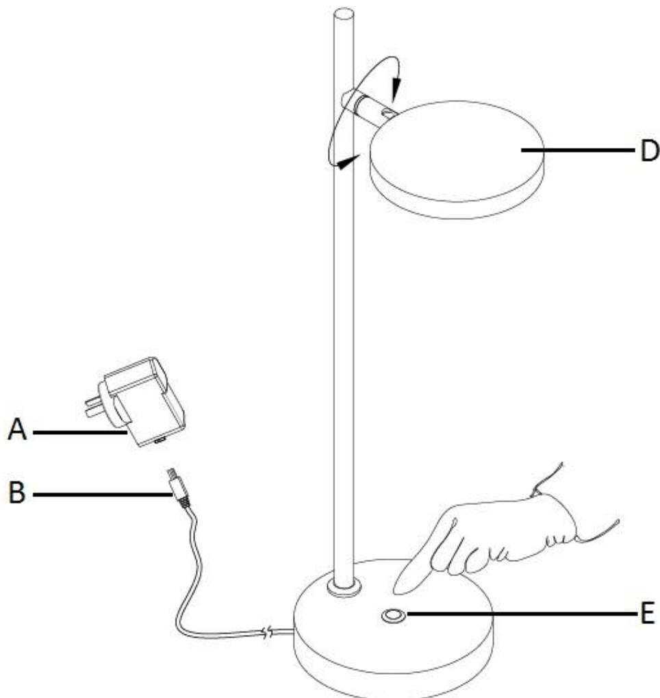
**NOTE:** When adjusting the head (D), do not adjust more than 360° as this may damage the internal wires.
