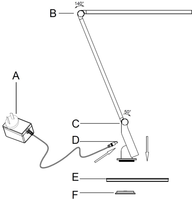
**NOTE:** When adjusting the upper arm, do not bend the joint (B) more than 140° as this may damage the internal wires.
